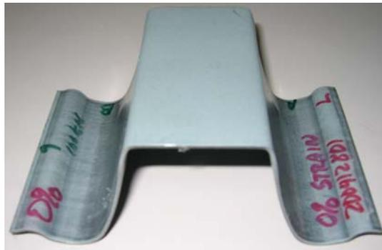
Fig. 9 A picture of the formed DP600 U-channel showing springback
